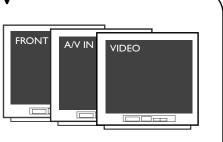
• If you only have a single antenna jack on the TV, you will need an RF modulator to connect the Receiver to your TV. The RF Modulator converts the Video from the Receiver so it can play through the TV's Antenna connector. When using an RF Modulator, you view DVD playback on TV channel 3 or 4 (like a VCR).
