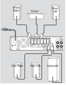
Connect the supplied speaker systems using the fixed speaker cables by matching the colors of the jacks and speaker cables.
