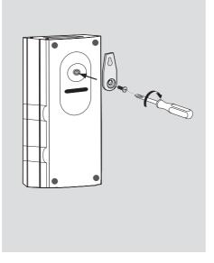
You can choose to mount the speakers on the wall. Attach the supplied bracket firmly to the rear of speakers using the supplied screws. Then mount a screw (not supplied) on the wall where the speaker is to be hung and hook the speaker securely onto the mounted screw.
