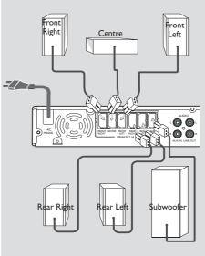
Connect the supplied speaker systems using the fixed speaker cables by matching the colours of the jacks and speaker cables.
