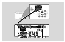
Before starting operation, press **AUX1/2/TV** on the remote control to select "TV" in order to activate the input source. The music will be heard through the speakers.
