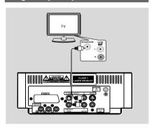
To listen to TV channels through this system, use the audio cables (white/red, not supplied) to connect AUX IN1 (L/R) jacks to the HEADPHONE jacks on the TV set (with a 3.5mm-diameter stereo jack).
