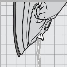
**1** Make sure the appliance is unplugged and set the steam control to position 0.
