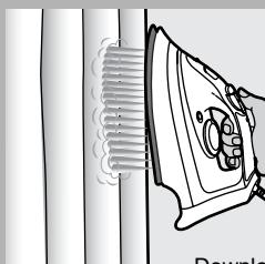
**1** The shot-of-steam function can also be used when you hold the iron in vertical position.
