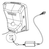
3 Connect the other end of the AC adaptor to the wall outlet.
