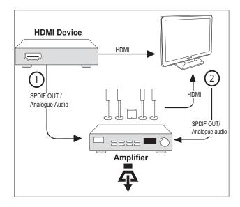
• Amplifier with one HDMI input and several HDMI outputs. Audio can be played by the amplifier via HDMI connector from your device.
