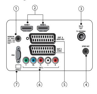
1 PC IN (VGA and AUDIO IN) Audio and video input from a computer.
