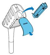
2 Insert 3 × AAA batteries (supplied) into the cartridge with correct polarity (+/-) as indicated.
