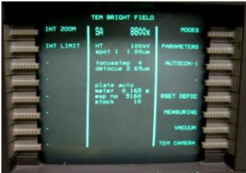
Figure 6 The main menu screen of the CM12 TEM
