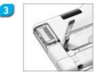
Put the Wireless LAN Adapter in the correct position until it clicks and close the cover.
