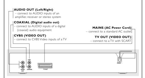
Caution: Do not touch the inner pins of the jacks on the rear panel. Electrostatic
