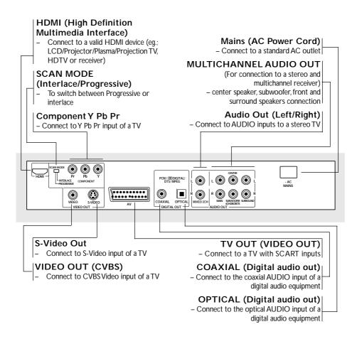
Caution: Do not touch the inner pins of the jacks on the rear panel. Electrostatic discharge may cause permanent damage to the unit.
