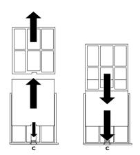
7 Insert the filter holder into the projector until it clicks in position...
