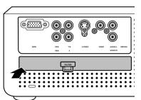
We advise you to clean the filter every 100 hours. Operating the projector without filter or with a torn or damaged filter may seriously damage the projector.
