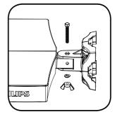
2 Use the screw holes of the wall/mast bracket ③ as a guide to mark position for the wood screws.
