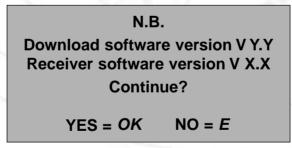
**f)** After pressing the **OK** key, the software version is checked. If the data carousel contains an older version, a message is displayed - if necessary you can interrupt download prematurely.
