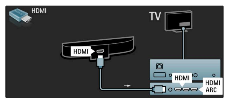
If you use the HDMI-ARC connections on both TV and device, no other cable is needed. If not, read on.
