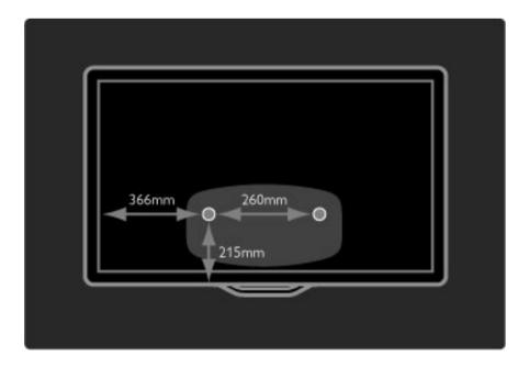
Fix the 2 mounting discs. Use screws with a diameter of max 6mm.
