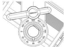
An additional tilt locking clamp can be added to the other side of the yoke if required (code: SPXTLOKIT). To fit, remove the yoke bolt cover with a flat blade screwdriver, and undo the M8 yoke bolt with a 13mm / ½" socket wrench. Gently lever open the yoke slightly and insert the cup head bolt in the yoke lock off hole. Add the spring and washer from the kit and then the locking clamp. Retighten the M8 yoke bolt, taking care to avoid over tightening, and replace the yoke bolt cover.
