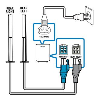
Connect the rear left and rear right speakers to the matching connectors at the back of the wireless receiver.
