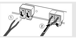
• Fully insert the stripped portion of the antenna into the terminals as shown.
