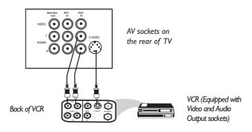
The S-Video connection on the rear of the TV is used for the playback of S-VHS VCR tapes, Video Discs, Video Games or Compact Disc-Interactive (cd-i) discs. Better picture detail and clarity is possible with the S-Video playback as compared to the picture from a normal antenna (RF) connection.
