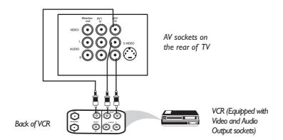
You can view the playback of VCR tapes (Video Disc players, camcorders, etc.) by using the AUDIO and VIDEO INPUT sockets on the rear of the TV.
