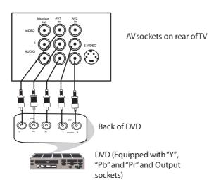
You can view the playback of DVD discs by using the COMPONENT VIDEO INPUT sockets on the rear of the TV.
