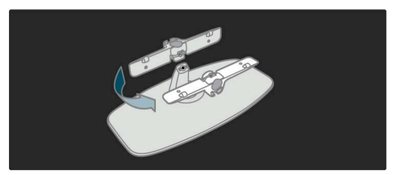
Reposition the bar on the stand and fix the bolt with the hex key.
