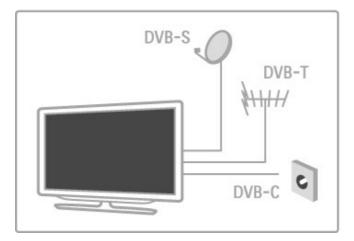
Next to the DVB-T and DVB-C reception, this TV has a built-in satellite DVB-S/S2 receiver. You can connect a satellite dish antenna and receive digital satellite channels.
