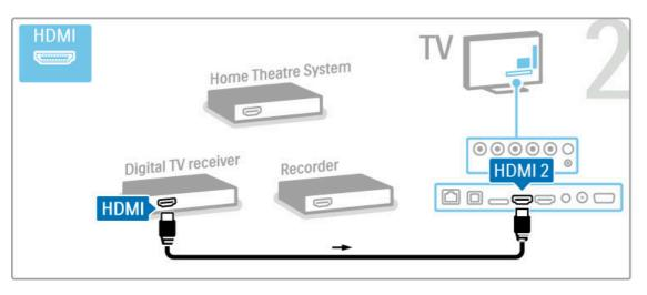
Then use an HDMI cable to connect the Disc Recorder to the  ${\sf TV}$
