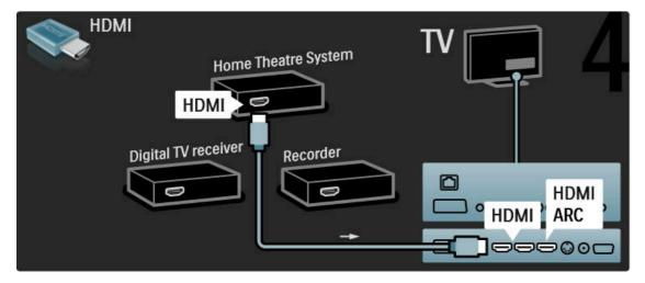
If you do not use the HDMI-ARC connection on the TV and the device, add a digital audio cable (cinch coaxial).
