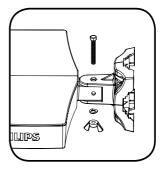
2 Insert U-bolts ③ into the holes of the wall/mast bracket ③. Slide the mast clamps ⑥ onto the U-bolts ⑤. Attach the four nuts with lock washers ⑦ to the U-bolts ⑤.
