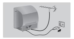
• Insert the aerial plug into the Tr socket at the rear of the set.
