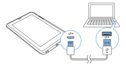
Do the following to transfer applications or media files from your PC to **Tablet 7**,the internal memory or SD card:
