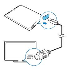
Connect an HDMI cable (sold separately) to: the HDMI socket on Pi7000, and the HDMI input socket on the TV.
