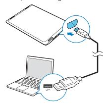
Connect Pi7000 to a PC by using the USB cable.
