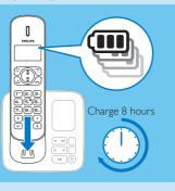
Place the handset on the base station to charge the handset. When the handset is placed correctly on the base station, you hear a docking sound.
