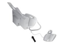
We recommend direct connection to the device because this allows the fax switch to function optimally and to control the additional devices.
