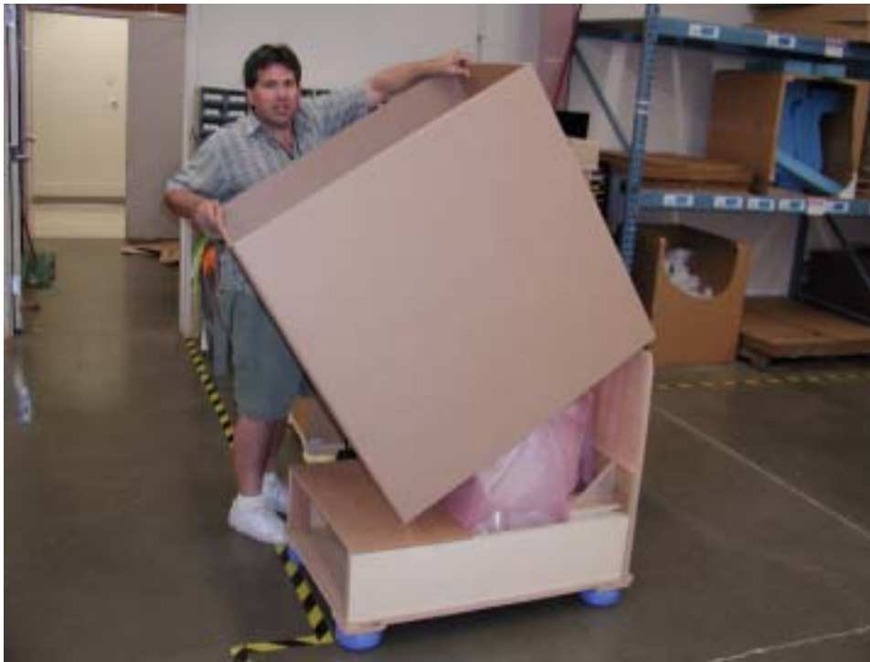
Figure 5-4 Removing the Corrugated Wrap
