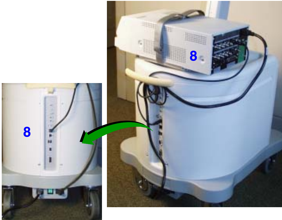
Figure 5-22 Cabling the Color Printer to the HD3 System
