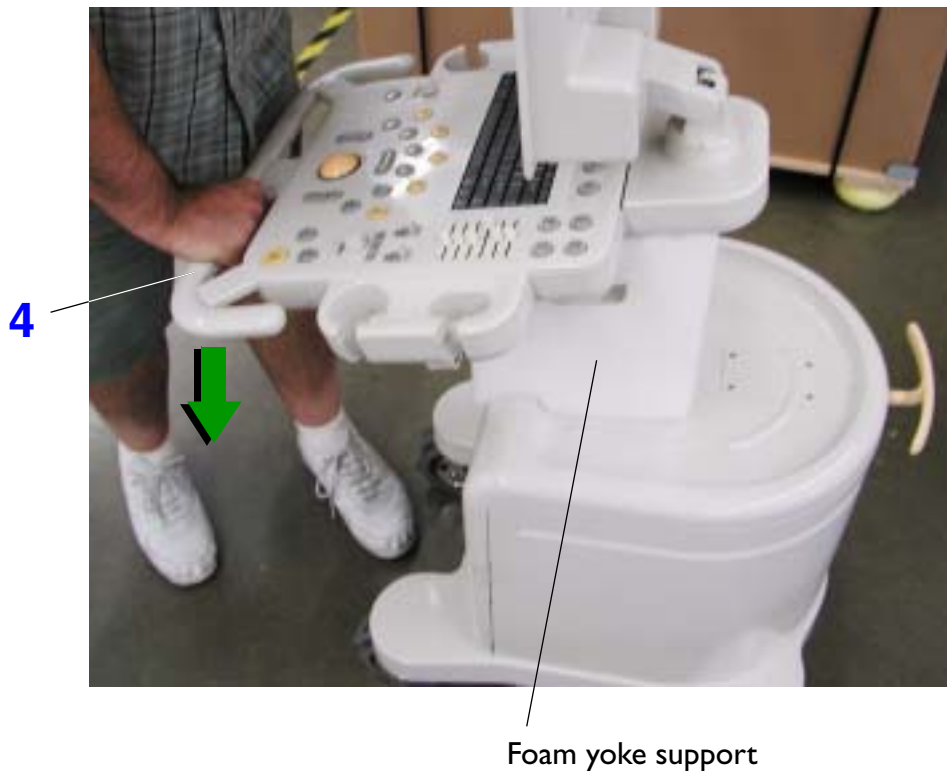
Figure 10-56 Lowering the Control Panel
