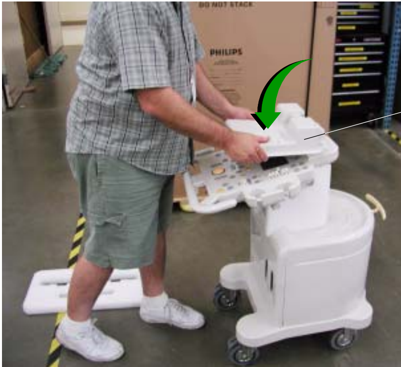
Figure 5-14 Tilting the Video Monitor
