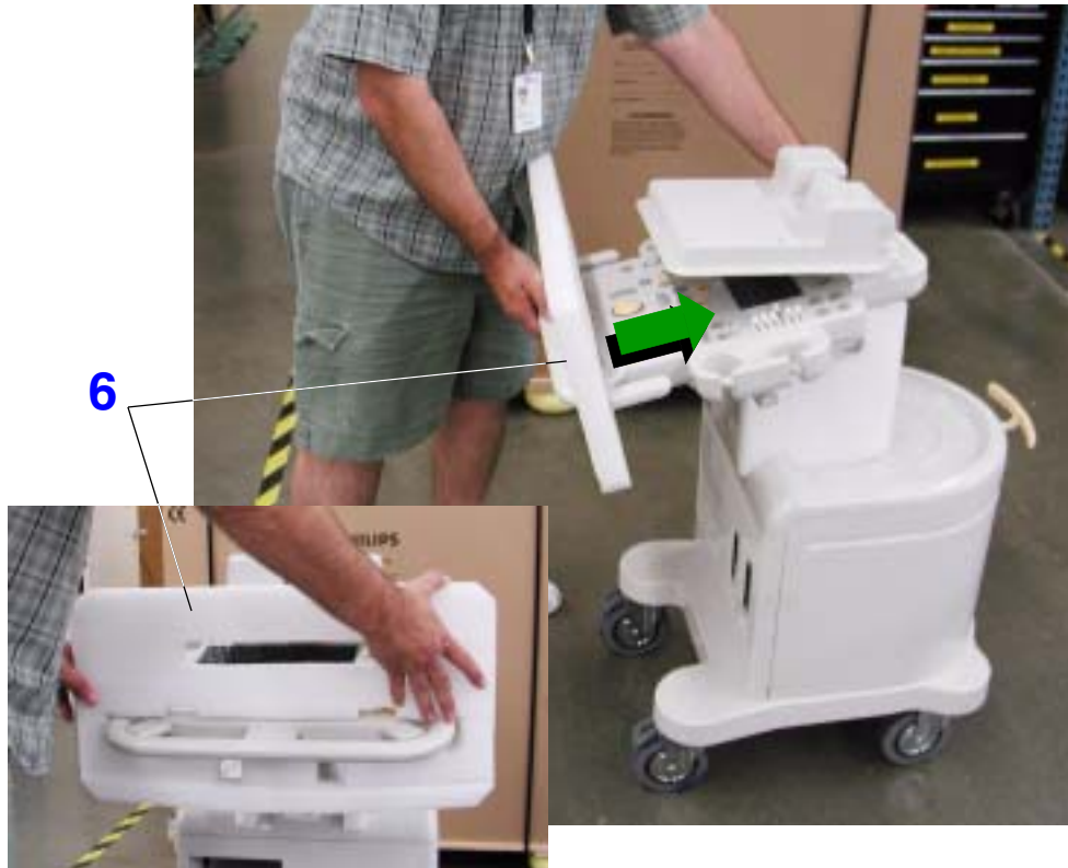
Figure 10-58 Placing the Foam Monitor Support
