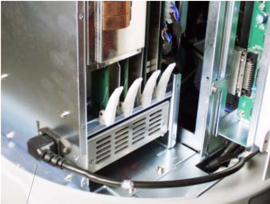
Figure 10-41 Disconnecting the Power Supply Power Cord
