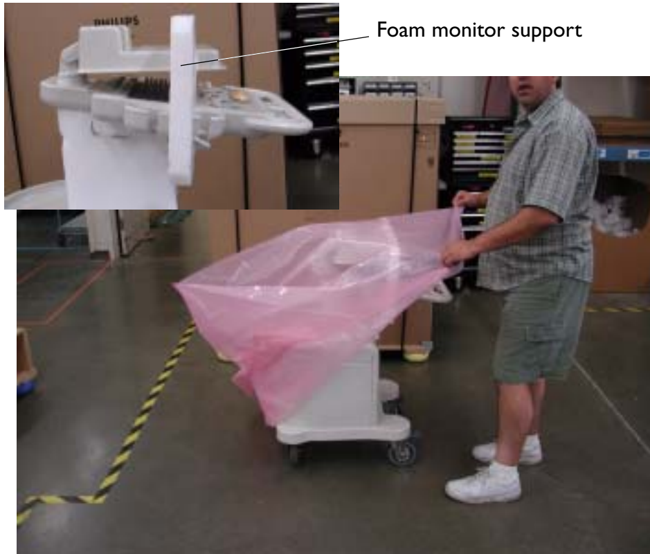
Figure 5-1 I Removing the Shipping Materials (Antistatic Bag and Monitor Support)
