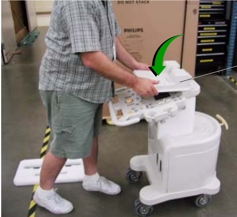
Figure 10-57 Tilting the Video Monitor
