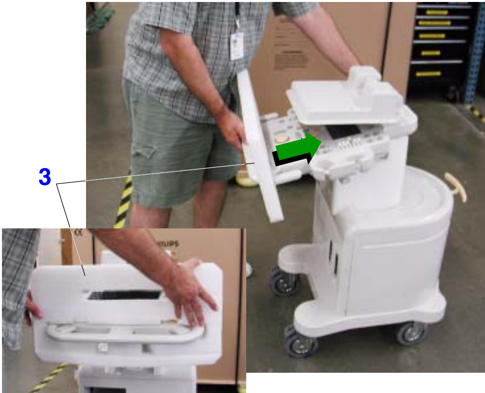
Figure 5-15 Placing the Foam Monitor Support
