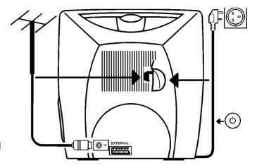
1 Insert the aerial plug into the  $\Box \Gamma$  socket.
