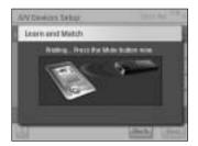
2 On the original remote control, press the button indicated by the RC9800i. Keep it pressed until the RC9800i indicates that it has learned the remote control code (or that it was unable to learn the code). Choose **Skip** if your original remote control doesn't feature the command asked for by the RC9800i.
