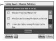
3 Choose Next and follow the on-screen instructions to configure all the activities you have selected. This means indicating which devices are involved in an activity, what A/V inputs are being used and, if applicable, what channels the device(s) must tune to.
