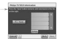
6 Choose Input to make the TV switch to an input. Indicate whether your TV shows the signal from its tuner (i.e. broadcasted programs) or an input. Repeat this step until all inputs, including the TV's internal tuner, have been added.
