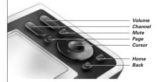
After you have properly set up the RC9800i, you can use the hard keys for the following functions:
