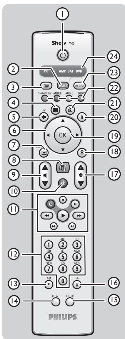
Note: When a key or key combination is pressed for longer than 30 seconds, the remote control will stop transmitting IR signals.
