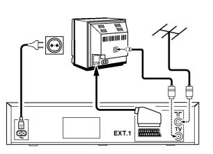
Remove the aerial cable plug from your TV set and insert it into the socket at the back of the video recorder.
