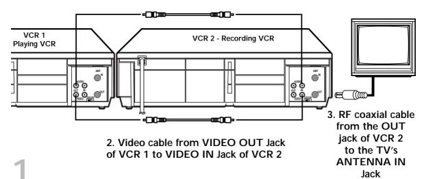
VCR 1 will play your tape. Insert a prerecorded tape in VCR 1. If the tape does not have a record tab, playback begins. If this happens, press the STOP/EJECT button on VCR 1 once.
