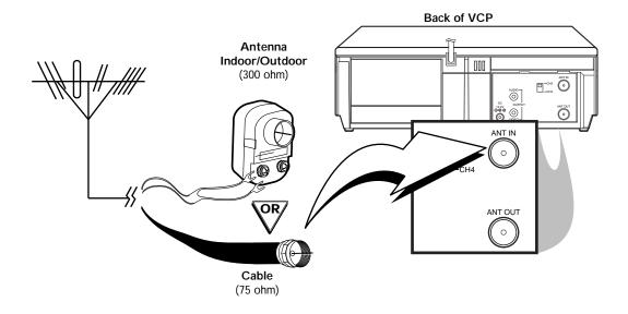
Connect the RF coaxial cable (supplied) to the ANT(enna) OUT jack on the back of the VCP and to the ANTENNA IN Jack on the TV. (You may use either a snap-on type or screw-on type of coaxial cable, whichever you prefer. A snap-on type is supplied.)
