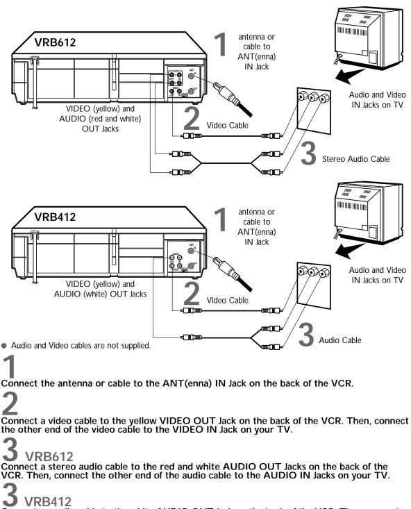
Connect an audio cable to the white AUDIO OUT Jack on the back of the VCR. Then, connect the other end of the audio cable to the AUDIO IN Jack on your TV. (If your TV has Right and Left AUDIO IN Jacks, you must use a "Y" splitter audio cable as illustrated to deliver audio to the TV's right and left channels.) This hookup will not give you stereo sound. To get stereo sound, use the connections on pages six - seven and select the channel to be viewed at the TV (with the VCR turned off).
