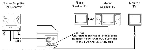
For stereo sound, connect the audio cables to the AUDIO OUT Jacks on the VCR and to the AUDIO IN Jacks on the Stereo Amplifier or Receiver. Then, connect the video cable to the VIDEO OUT Jack of the VCR and to the VIDEO IN Jack of a monitor TV.
