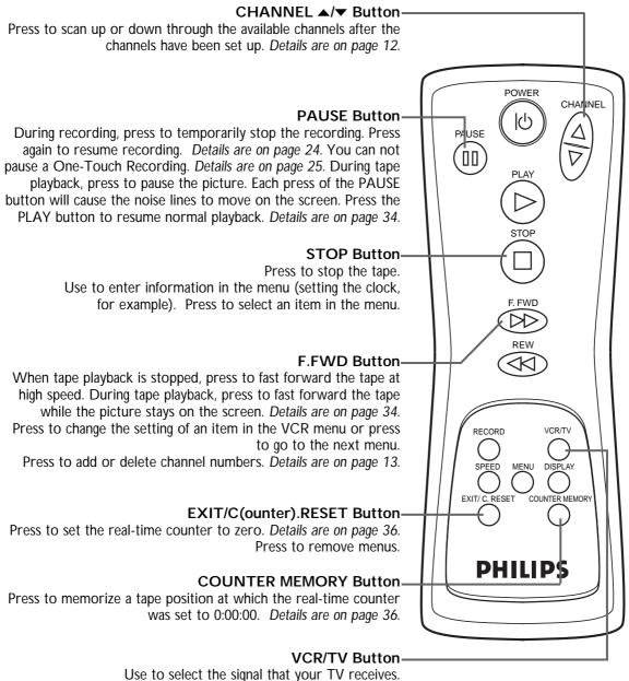
Use to select the signal that your TV receives. • VCR Position Use to watch a tape, to watch a program while recording it, or to
