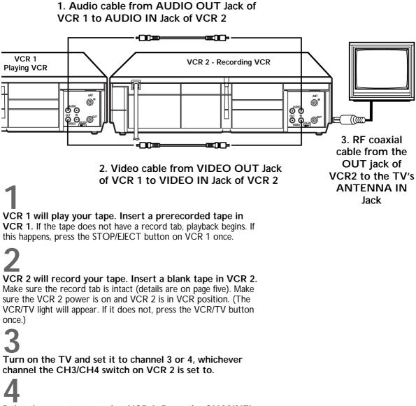
Point the remote control at VCR 2. Press the CHANNEL ▲/▼ buttons until LineIn Rear (L1) appears on the screen.
