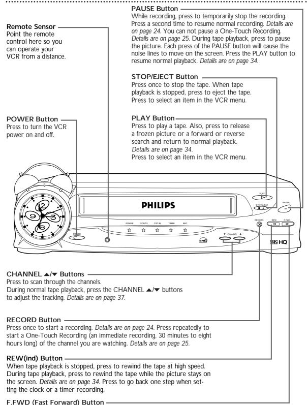
When tape playback is stopped, press to fast forward the tape at high speed. During tape playback, press to fast forward the tape while the picture stays on the screen. *Details are on page 34.* Press to select an item in the VCR menu or to change the setting of an item.
