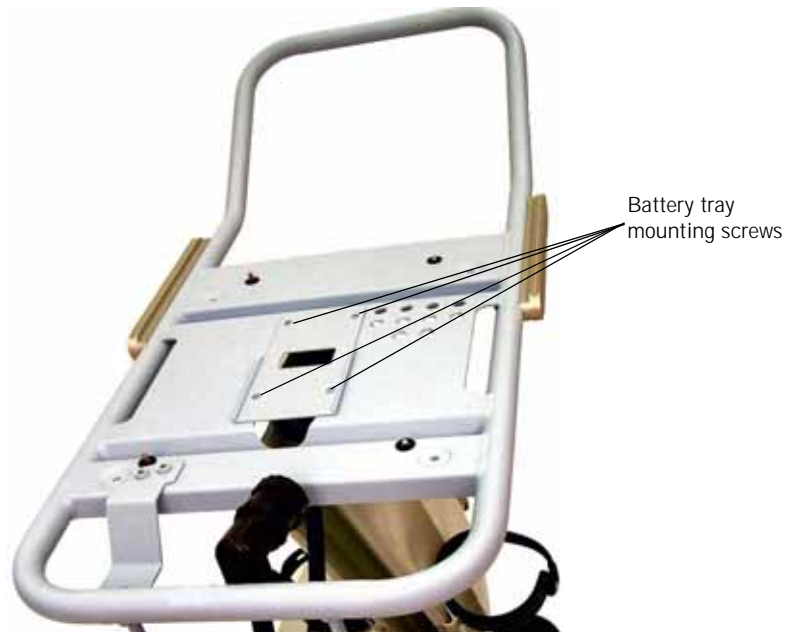
Figure 4-7: Removing the Battery Tray
