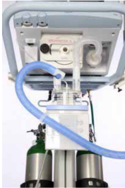
Figure 6-6: Humidifier Outlet to Patient Wye Connection
