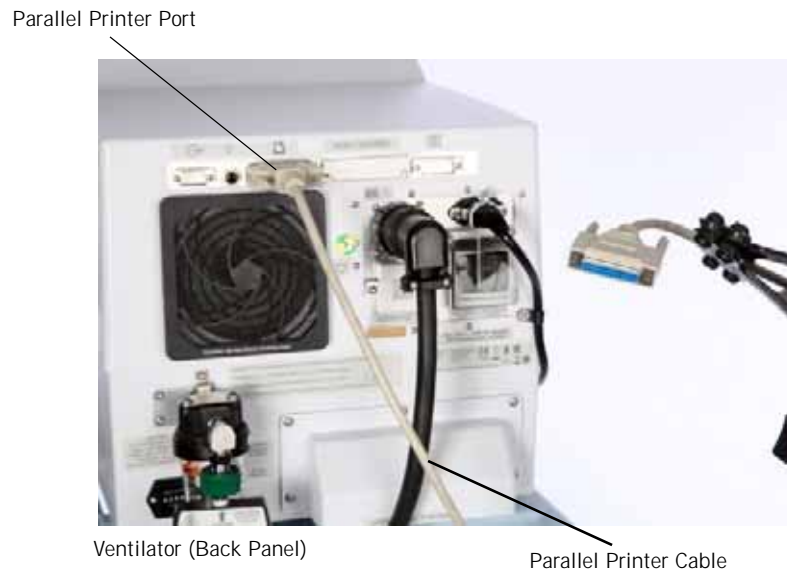
Figure 13-24: Connecting the Ventilator to a Printer
