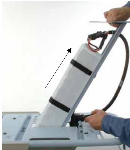
Figure 4-8: Removing the Battery Tray
