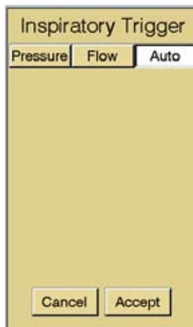
Figure 13-73: Sample Inspiratory Trigger Window with Auto-Trak Option Selected (Pressure is not an available option for NPPV)
