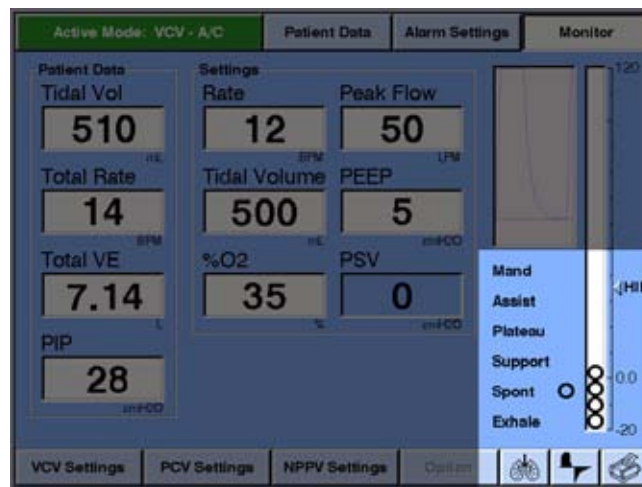
Figure 13-42: Breath Indicator During Flow-Trak Breath
