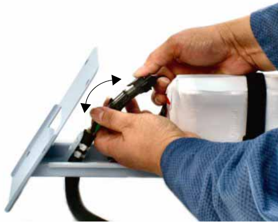
Figure 4-9: Disconnecting the Old Battery from the Battery Tray's Cable
