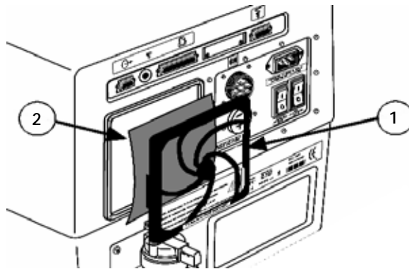
Figure 10-4: Removing Cooling Filter
