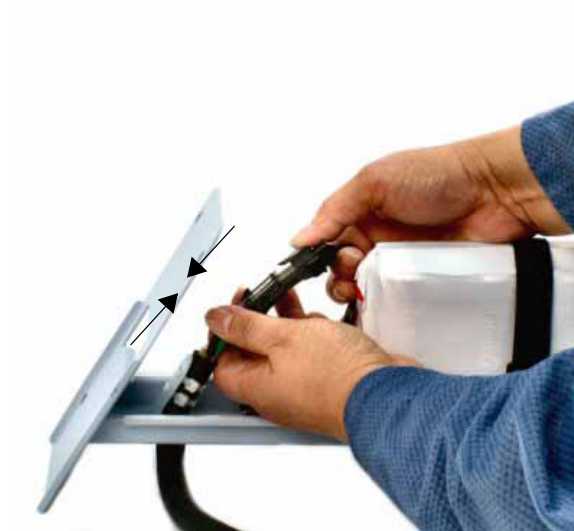
Figure 4-12: Connecting the Battery to the Battery Tray's Cable
