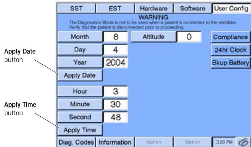
Figure 5-9: User Configuration Screen After Date and Time are Set
