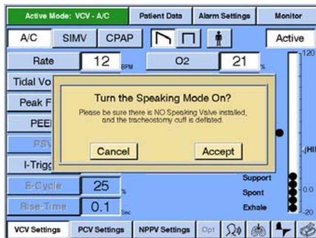
Figure 13-61: Turn the Speaking Mode On? Reminder Second Message Box
