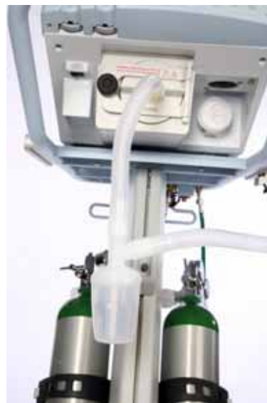
Figure 6-7: Expiratory Limb of Patient Circuit to Water Trap Connection (Shows Down Tube between Ventilator and Water Trap)
