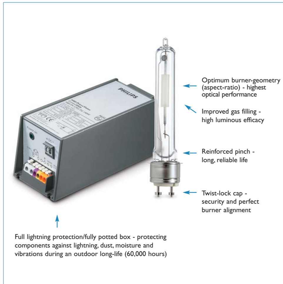
65% smaller than SON and HPI/CDO lamps - design flexibility for small, high-performance luminaires
