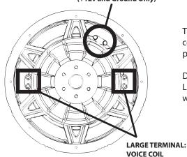
The Elite.12 has three terminals. The two larger terminals are connected to the voice coils. The small terminal is used to power the LEDs with a +12v and ground connection only.
