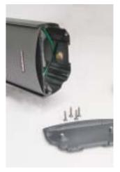
Find a pair of wires with slide-on connectors loose in the bottom of the AST 220S. These will mate with the two wires extending from the AST-Stands.
