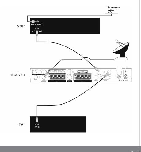
3.4 Connecting to TV and VCR using RF Support and RCA
