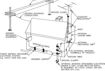
provide some protection against voltage surges and built-up static charges.
