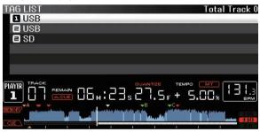
When multiple storage devices (SD, USB) are connected to the DJ player, the number of the player to which that storage device (SD, USB) is connected is displayed in front of the storage device's (SD,
