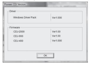
The firmware version is not displayed when this unit is not connected to the computer or when this unit and computer are not properly communicating.
