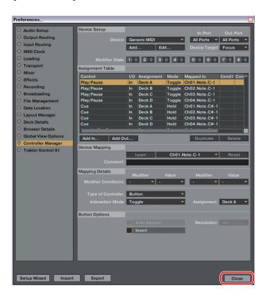
The above settings will allow you to control TRAKTOR PRO/PRO 2 from the Multi Player machine. If you will use the Multi Player as a TRAKTOR PRO/PRO 2 audio output device, see the "Using Multi Players as TRAKTOR PRO/PRO 2 Audio Output Devices" on page 12.
