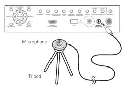
If you have a tripod, use it to place the microphone so that it's about ear level at your normal listening position. If you do not have a tripod, use some other object to install the microphone.<sup>1</sup>
