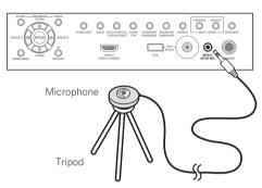
If you have a tripod, use it to place the microphone so that it's about ear level at your normal listening position. If you do not have a tripod, use some other object to install the microphone.<sup>3</sup>
