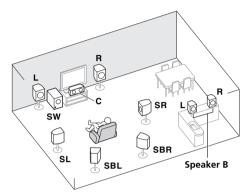
With these connections you can simultaneously enjoy 5.1-channel surround sound in the main zone with stereo playback of the same sound on the B speakers. The same connections also allow for 7.1-channel surround sound in the main zone when not using the B speakers.
