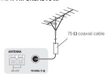
To improve AM reception, connect a 5 m to 6 m (16 ft. to 20 ft.) length of vinyl-coated wire to the  $\bf AM\ LOOP$  terminals without disconnecting the supplied AM loop antenna. For the best possible reception, suspend horizontally outdoors.
