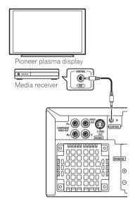
Use a 3-ringed miniplug SR+ cable to connect the CONTROL IN jack of this unit through a media receiver to the CONTROL OUT jack of your plasma display.
