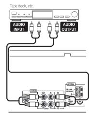
Connect the LINE 1 (IN) jacks to the analog outputs of an external playback component.
