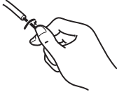
1: Strip the cover and twist the strands
